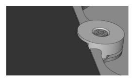
Multi-Step Retainer Orientation for Securing a Filter with <u>5 mm</u> Thickness
