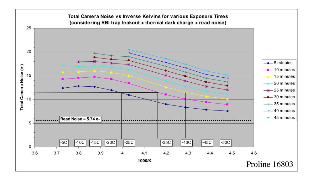
$$Total\_camera\_noise = \sqrt{(trap\_leakage + thermal\_dark\_signal) + read\_noise^2}$$
