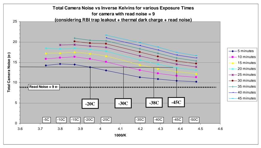
$Total\_camera\_noise = \sqrt{(trap\_leakage + thermal\_dark\_signal) + read\_noise^2}$
