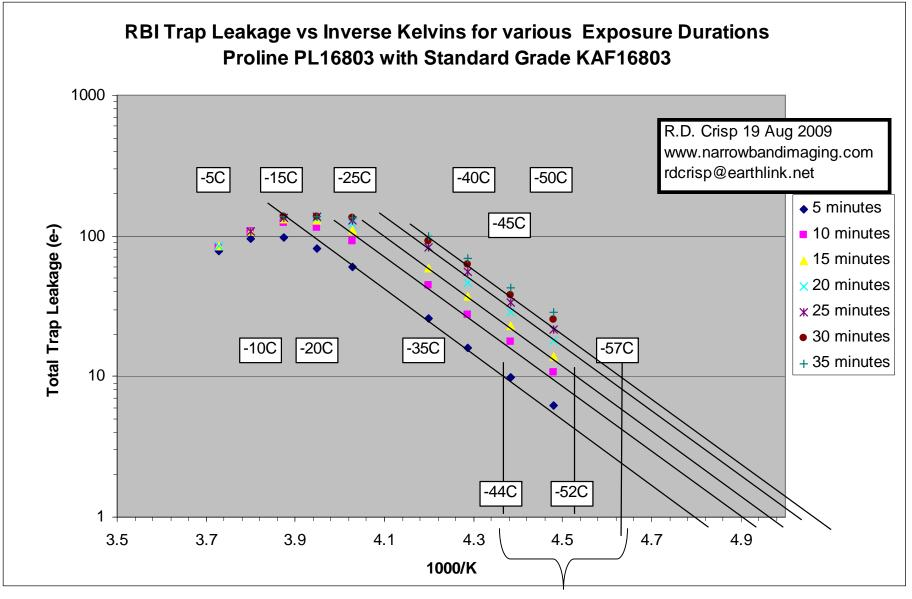
Measured Capacity RBI Traps: ~140 erdcrisp@earthlink.net 10e- RBI Trap leakage reached 5 minutes @ -44c 15 minutes @ -52C 30 minutes @ -57C 23 Aug 2009
